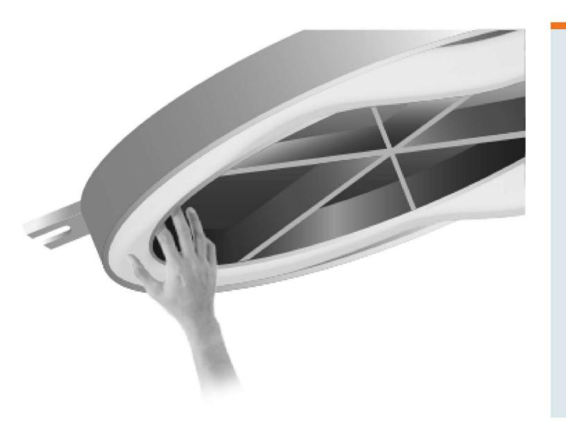
4. For toggle hatches use the sequence shown when tightening, this ensures even distribution of load/compression, helping to prevent leaks.
